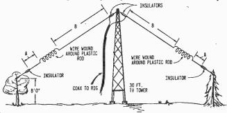
W7DQS made use of a 30-ft. TV mast and a couple of trees to support his 80/40 doublet, but your instaltion needn't be the same. Lengths A and B were 4 ft. 6 in. and 35 ft. 10 in. in his case — exact dimensions must be determined through use of an SWR bridge as described in text.
