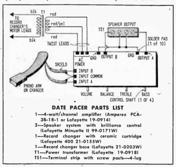
pads, pre-tinned spots on the printed-circuit board approximately 1/4-in. square.
