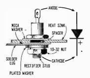
Above, mounting details for diodes D1-D4. Below, Spender with its cover removed.
