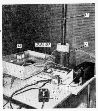
Completed Lightning Generator stands ready to go with all of a million volts! Wiring between components is AWG-12 or 14.
