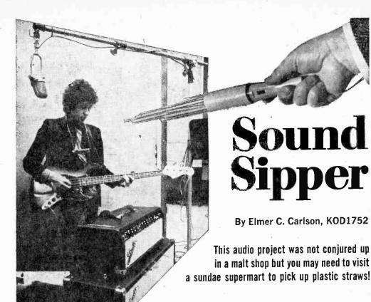
They're free! That's right! All the basic materials needed for making a lightweight directional baffle for your recorder's microphone are free. All you need is a handful of plastic drinking straws, a plastic sleeve and a few small rubber bands, and voila-Sound Sipper,
