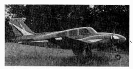
Newly developed Copsul light on aircraft permits pilots to see a plane's shape up to three miles away in dusk and darkness. Picture of above aircraft was taken in early evening. Strips of Capsul are on tail, mid-fuselage, wing tip and engine cowling make in-the-air sightings easy.
