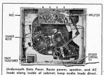
the schematic diagram.) Staple, tape or cement the wires to the inside of the base.
