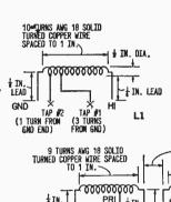
Drawings at left and below give full details for winding coils L1 and L2; see photo on next page for placement of secondary winding on L3. Location of components on perf-board can also be seen on this photo as well as on the pictorial below.
