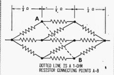
Now, all resistors fall into one of three parallel groups that are in series with other groups. The first group on the left consists of three one-ohm resistors, which effectively add up (or is it down, in this case?) to  $\frac{1}{3}$  ohm. The same summation is true for the group on the right. The center group consists of six resistors and sums to  $\frac{1}{3}$  ohm. Hence, when you add up  $\frac{1}{3} + \frac{1}{3} + \frac{1}{3}$ , the answer comes to  $\frac{5}{6}$  ohm.
