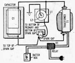
Pictorial diagram of Lightning Generator. Leads are attached directly to tabs on C1.
