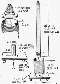
Platform for coil L2 is made from  $9 \times 9$  in. square of  $\frac{1}{2}$ -in. plywood.
