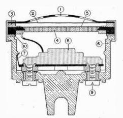
A cross-sectional view of the electret transmitter showing (1) screen, (2) dust and humidity cover, (3) contact spacer, (4) perforated back plate, (5) electret diaphragm, (6) cup, (7) contact spring, (8) amplifier assembly, (9) screw terminols and (10) contact ring. This new electret microphone fits directly into the present telephone handset with no modifications.
