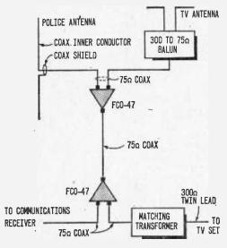
47 through the same kind of coax and a 75-ohm to 300-ohm matching transformer. All connections to the FCO-47's must be made with suitable coax connectors. The FCO-47 (available from Jerrold Electronics, 401 Walnut Street, Philadelphia) passes signals from 5 to 47 MHz (Continued on page 133)
